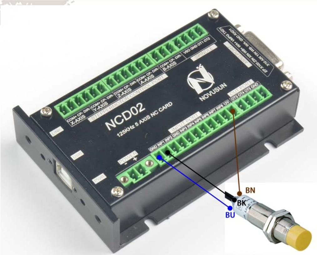
Figure2-7. NPN 3 line Proximity switch wiring
